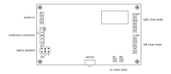
The board is designed to be powered either from a 6.3v AC supply (typical heater supply will be ideal, but check it is not a higher voltage), or a 9v DC supply. The polarity of the supply is not important.
