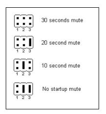
As supplied the board has all jumpers fitted which corresponds to no startup mute and no motor wind down.
