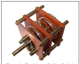
Figure 2. The 34-way Seiden Switch
