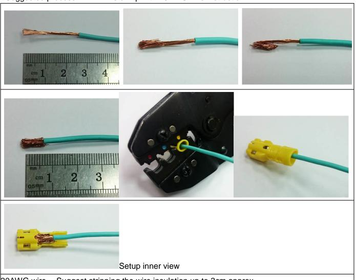
20AWG wire--- Suggest stripping the wire insulation up to 3cm approx.
