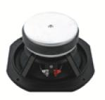
The B220.2 uses a symmetrical field magnet system with a long coil for large linear excursion capability. Double rear suspensions guarantee transient stability at high drive levels. The cone is doped for minimal colouration. The Thiele-Small parameters are optimised for easy use in relatively small enclosures to give extended bass performance.
