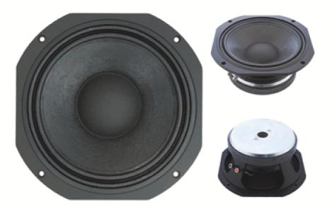
The BM2500.4 uses a massive magnet with a symmetrical field, extended pole and exceptionally long voice coil for maximum linearity. The cone, linen surround and dome are critically matched and doped to ensure very low midband colouration. The result is analytical sound quality with a stunning dynamic range.
