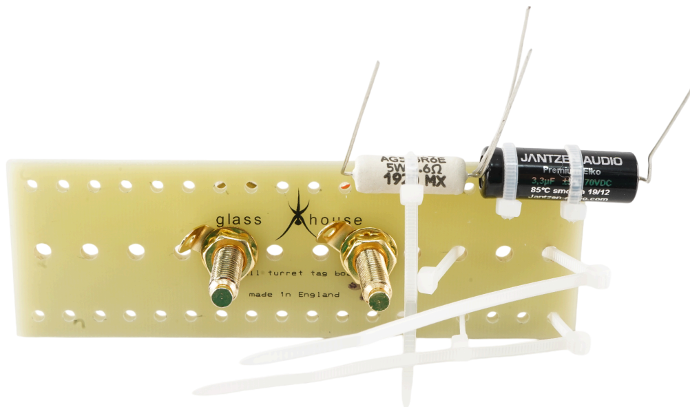
R1 and C1 attached to crossover board, tweeter section
