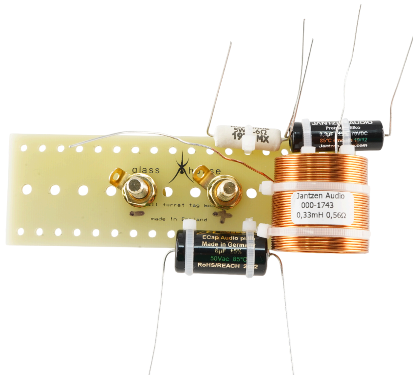
Tweeter section components attached
