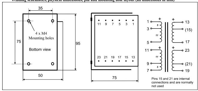
Weight: 1.35 kgStatic resistance of each primary:  $105~\Omega$ Static resistance of secondary (connected in parallel as below):  $0.4 \Omega$ Isolation between windings / between windings and core: 4 kV / 2 kV Max recommended DC current through any primary winding: 160mA
