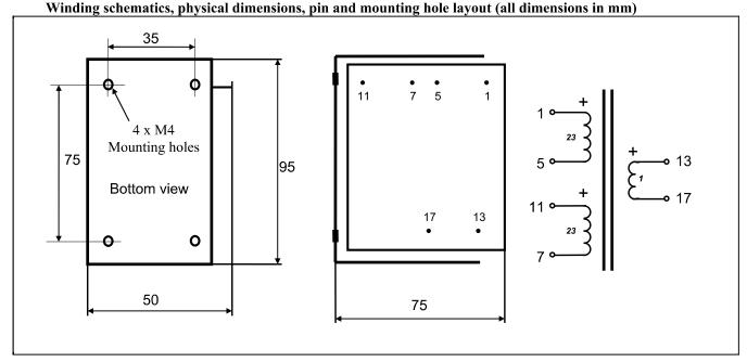
Weight:1.35 kgStatic resistance of each primary: $270 \Omega$ Static resistance of secondary: $0.2 \Omega$ Isolation between windings / between windings and core:4 kV / 2 kVMax DC current through any primary winding:100 mA (6W heat power)
