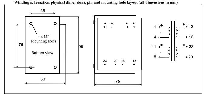
Weight: 1.35 kg Static resistance of each primary:  $75 \Omega$ Static resistance of secondary:  $290 \Omega$ Isolation between windings / between windings and core: 4 kV / 2 kV Max recommended DC current through any primary winding: 220mA (5W heat dissipation)
