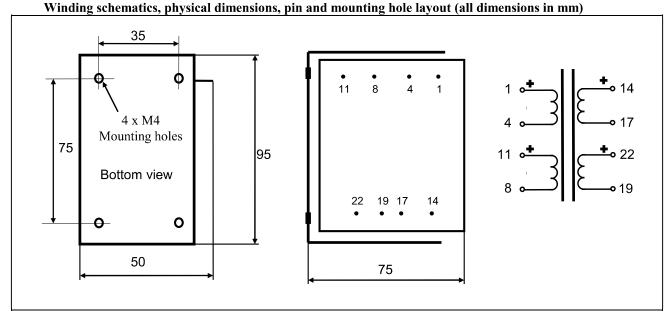
Weight: 1.35 kg Static resistance of each primary:  $75 \Omega$ Static resistance of secondary:  $75 \Omega$ Isolation between windings / between windings and core: 4 kV / 2 kV Max recommended DC current through primary windings: 180mA (5W heat dissipation)
