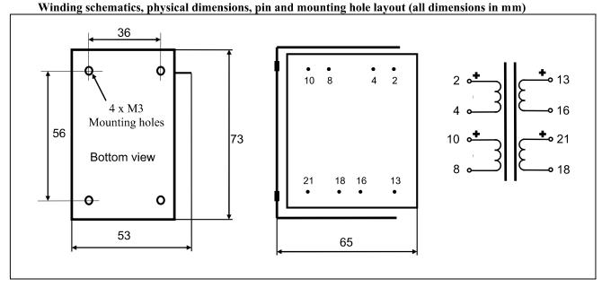
Weight:0.6 kgStatic resistance of each primary: $7 \Omega$ Static resistance of secondary: $7 \Omega$
