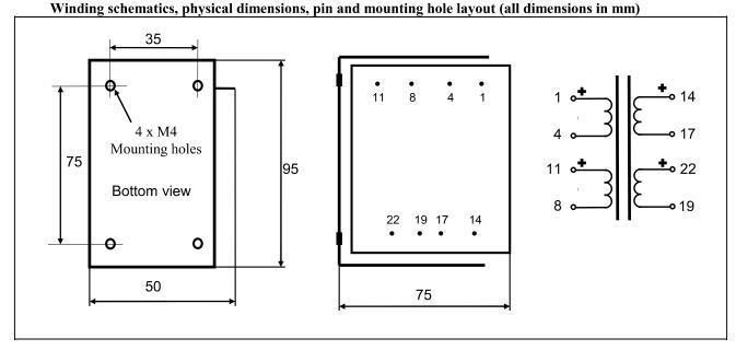
Weight: 1.35 kg Static resistance of each primary:  $180~\Omega$ Static resistance of secondary:  $180 \Omega$ Isolation between windings / between windings and core: 4 kV / 2 kV Max recommended DC current through primary windings: 120mA (5W heat dissipation)
